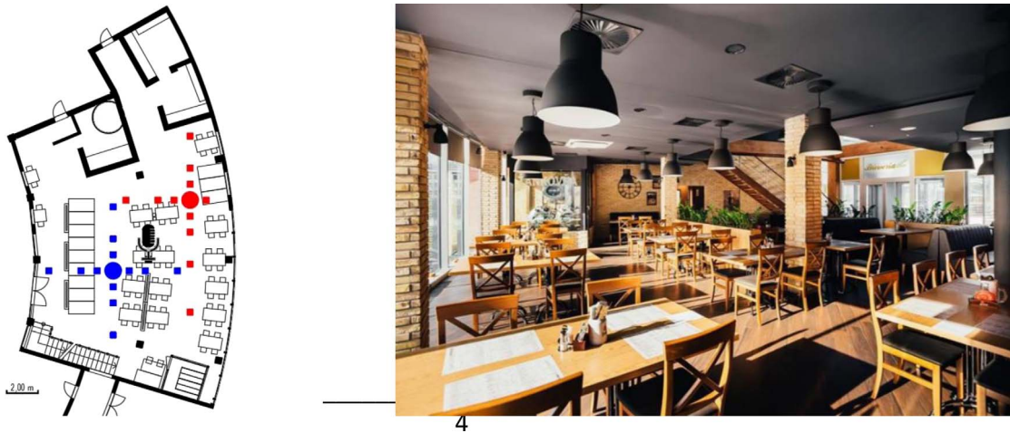
Figure 3. Floor plan (left) and photo (right) of restaurant Breweria 1, with indication of sound sources and microphone positions. Circles indicate sound sources, squares indicate microphones used during impulse response measurements, the black microphone indicates the position of the sound pressure level monitoring device.
