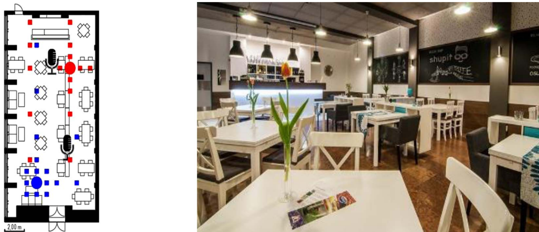
Figure 2. Floor plan (left) and photo (right) of Faculty Club Shupitoo, with indication of sound sources and microphone positions. Circles indicate sound sources, squares indicate microphones during impulse response measurements, the black microphone indicates the position of the sound pressure level monitoring device.
