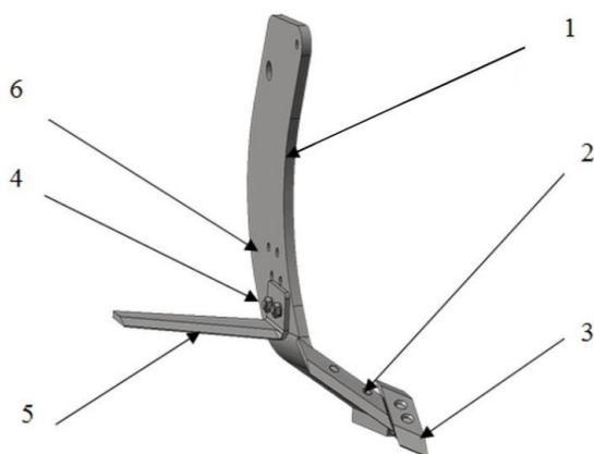
Fig. 1. Working body "ROPA": 1 - rack; 2- blade; 3- chisel; 4- fastening bolt; 5- paw; 6- attachment point of the trimming foot.
