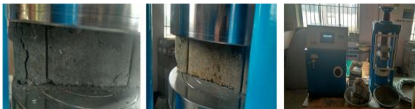
Fig. 4. Test on compressive strength of bricks
