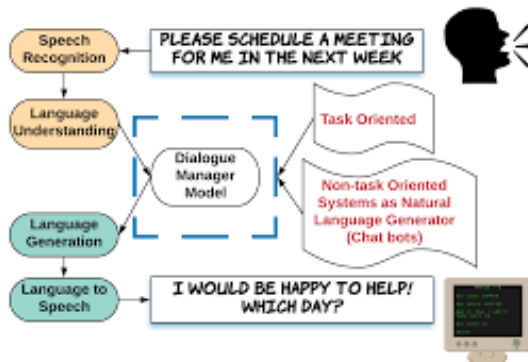
Figure 1: The working of a dialogue system
