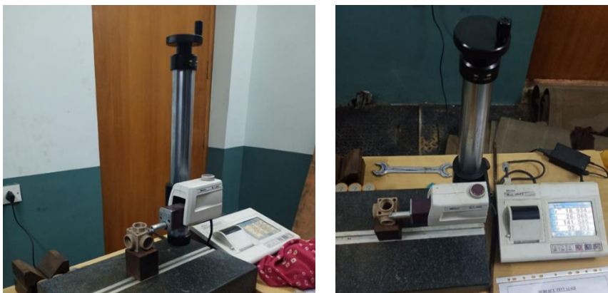
Fig. 2. Surface roughness testing machine (Mitutoyo SJ-410).
