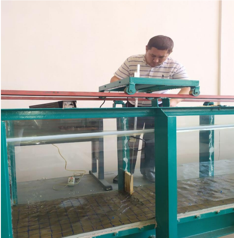
Fig. 1. Experimental studies of combined dam
