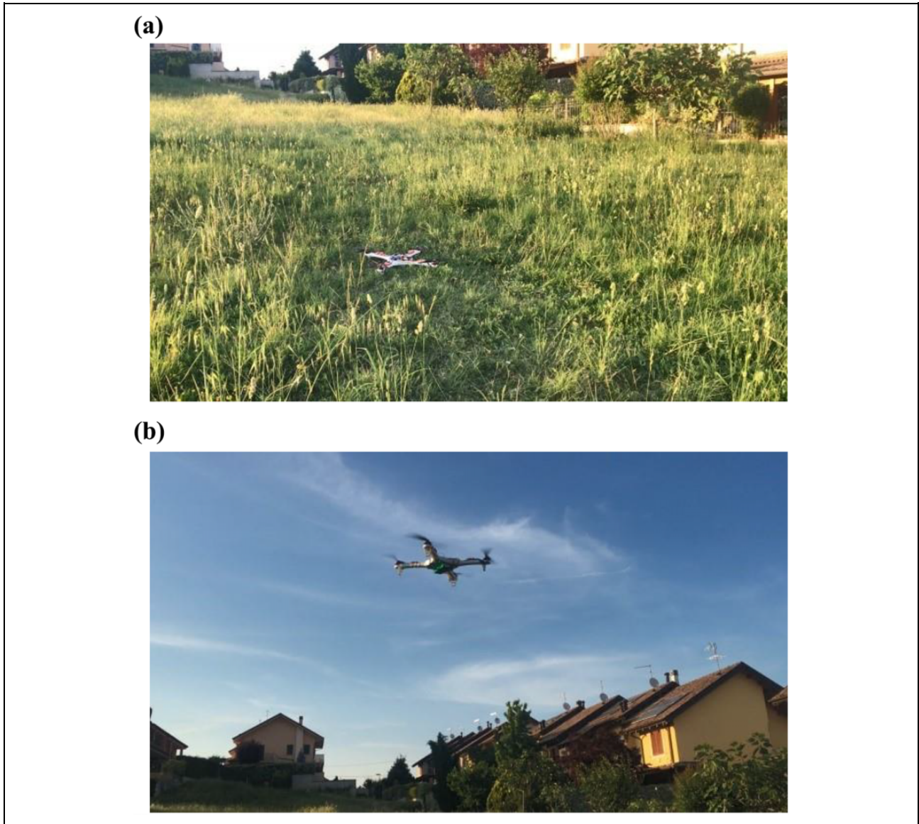
Figure 14. An outdoor test of the flight module of HBIII: (a) starting position; (b) stationary flight at a prescribed altitude of 8 m.
