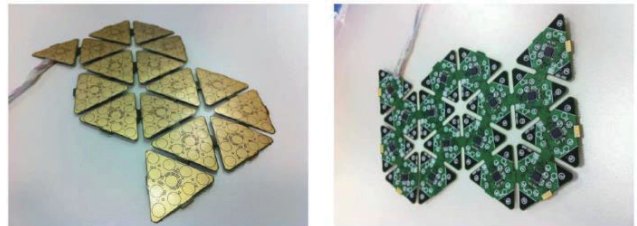
Fig. 2: the iCub skin solution; flexible PCB structure showing the sensor allocation (left) and connection routing (right).
