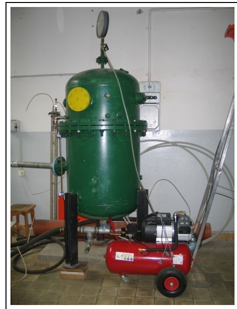
Figure 3. Pressure increasing station with the compressor.
