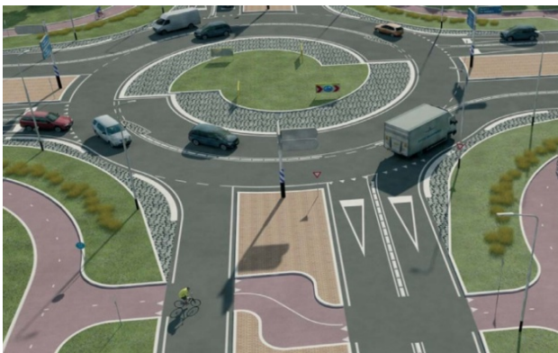
Fig. 2 Rendering of a turbo roundabout.
