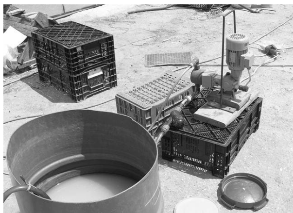
Fig. 2. Distribution system of agro-chemicals and biological control agent by sub-irrigation
