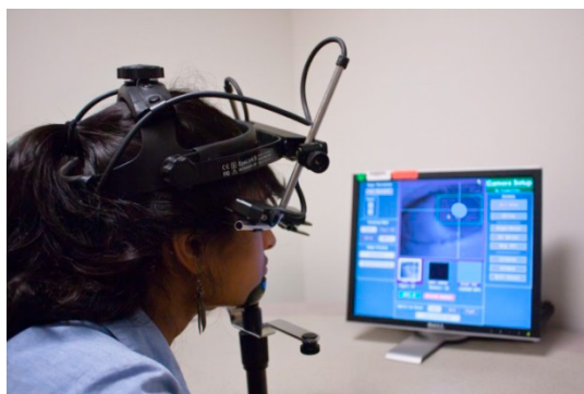
Fig. 4. Example of the usage of a video-based eye tracker.
