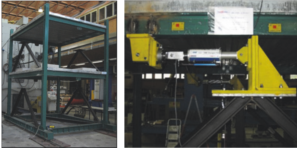
FIGURE 2: The experimental mock-up structure.
