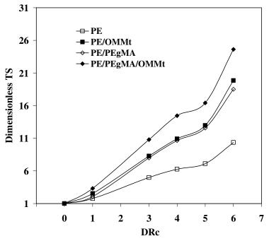
Fig. 5. Dimensionless tensile strength as a function of the draw ratio. The dimensionless values have been calculated by dividing the values of the fibres by those of the compression-moulded sheets. *Dintcheva N.Tz, Marino R, La Mantia F.P: The role of the matrix–filler affinity on morphology and properties of polyethylene/clay and polyethylene/compatibilizer/clay nanocomposite drawn fibres. e-Polymers. 2009, no. 054. Copyright e-Polymers. Reproduced with permission.*
