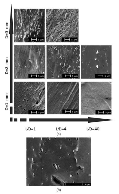
Fig. 4. SEM micrograohs of PE/OMMt fibres (a) considering capillaries with different geometries and compounded PE/OMMt sample (b). *La Mantia F.P, Marino R, Dintcheva N.Tz: Morphology Modification of Polyethylene/Clay Nanocomposite Samples under Convergent Flow. Marcomolecular Matererial and Engineering.* 2009, 294, 575-581, Copyright Wiley-VCH Verlag GmbH & Co. KGaA. Reproduced with permission.
