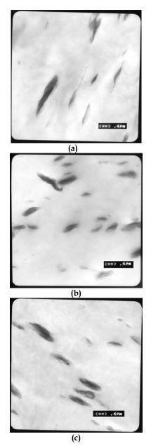
Fig. 3. TEM micrographs of (a) compounded PE/OMMt sample, (b) PE/OMMt fibre at DRc=1, (c) PE/OMMt fibre at DRc=6. La Mantia F.P, Dintcheva N.Tz, Scaffaro R, Marino R: Morphology and Properties of Polethylene/Clay Nanocomposite Drawn Fibre. Marcomolecular Matererial and Engineering. 2008, 293, 83-91, Copyright Wiley-VCH Verlag GmbH & Co. KGaA. Reproduced with permission.
