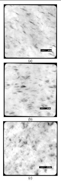
Fig. 6. TEM micrographs of (a) compounded PE/PEgMA/OMMt sample, (b) PE/PEgMA/OMMt fibre at DRc=1, (c) PE/PEgMA/OMMt fibre at DRc=6. Dintcheva N.Tz, Marino R, La Mantia F.P: The role of the matrix–filler affinity on morphology and properties of polyethylene/clay and polyethylene/compatibilizer/clay nanocomposite drawn fibres. e-Polymers. 2009, no. 054. Copyright e-Polymers. Reproduced with permission.
