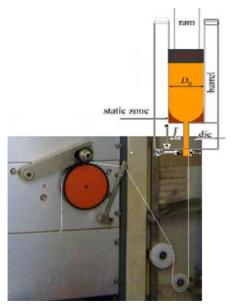
Fig. 1. Scheme of apparatus for filament formation
