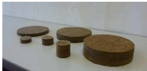
Fig. 2. Basalt fiber specimens for the acoustic experimental campaign.
