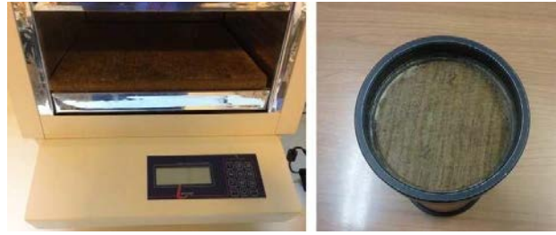
Fig. 3. Samples inserted in the experimental apparatus: heat flow meter apparatus (left) and Kundt's Tube (right).
