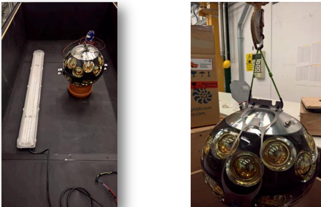
FIG. 6: set-up to measure the effect of illumination (left), the system to hold the DOM (right).
