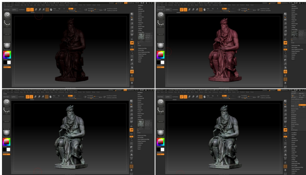
Figure 7. On the left, triangular model made up of 6 ML of triangular polygons. On the right, a retopologized model consisting of 57646 quadrangular polygons
