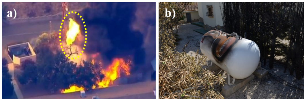
Fig. 1. (a) Calabassas fire (California, 2016 – credit KABC-TV). A propane jet fire can be observed at the center of the image (inside the yellow dotted ellipse). Flames from ornamental fuels are close to the tank. LPG infrastructure was inside a kindergarten; (b) Domestic LPG tank in Benitatxell (Spain, 2016 – credit D. Caballero) damaged by a jet fire from the PRV. The tank was surrounded by an ornamental hedgerow that ignited by spotting. (For interpretation of the references to colour in this figure legend, the reader is referred to the web version of this article.)
