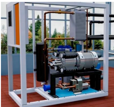
Figure 1. StarEngine micro-ORC installation at the well site
