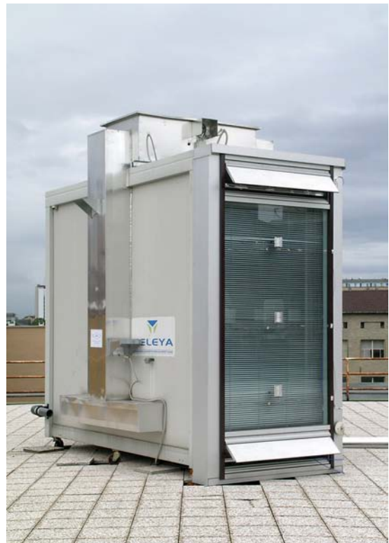
FIGURE 2. The DSF tested at the TWINS facility.
