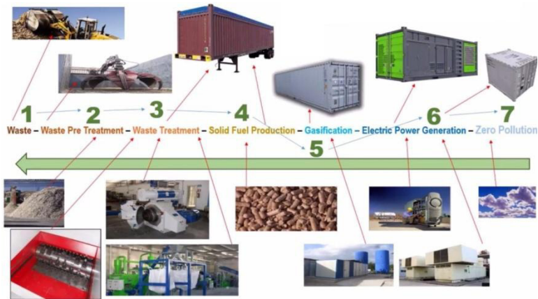
Fig. 2. Diagram of the integrated waste treatment platform with the innovative SRF production system.
