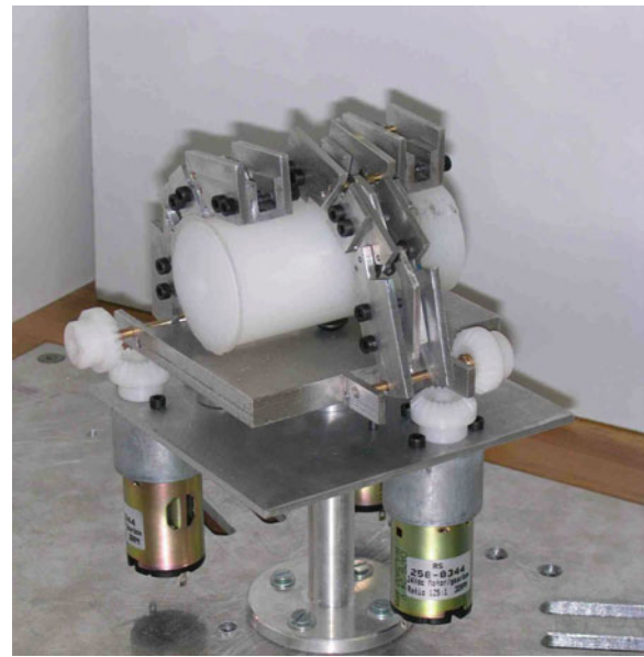
Figure 2 A prototype of three-fingered LARM hand with 1 d.o.f. anthropomorphic fingers of human sizes.
