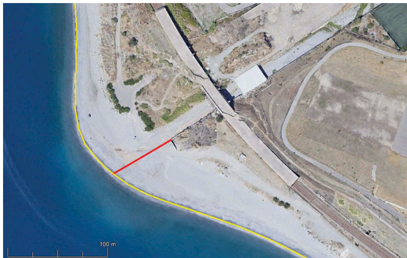
Figure 8. Shorelines of September 2017 and transept digitized using the spatial analysis tools of Google Earth Pro. Legend: yellow = shoreline, red = transept. (source: satellite imagery of Google Earth Pro).
