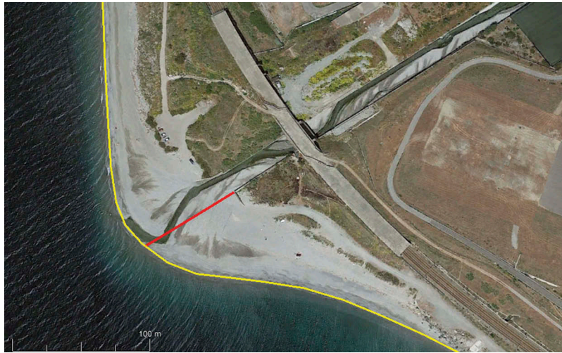
Figure 7. Shorelines of March 2015 and transept digitized using the spatial analysis tools of google earth pro. Legend: yellow = shoreline, red = transept. (source: satellite imagery of Google Earth Pro).
