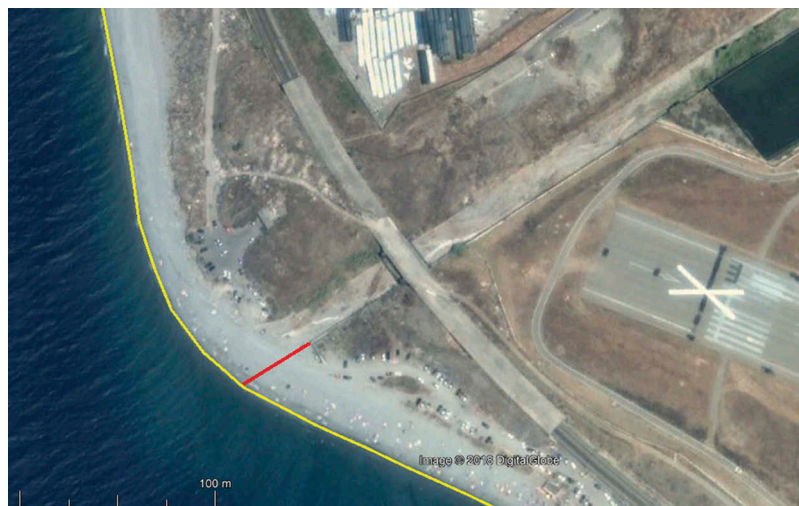
Figure 6. Shorelines of July 2007 and transept digitized using the spatial analysis tools of Google Earth Pro. Legend: yellow = shoreline, red = transept. (source: satellite imagery of Google Earth Pro).
