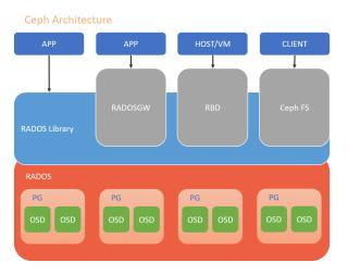
FIGURE 1: Ceph Architecture.
