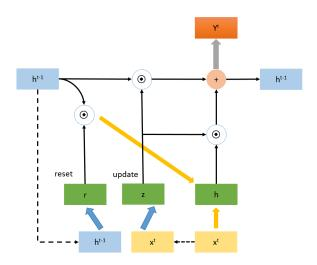
FIGURE 6: GRU Internal Structure.
