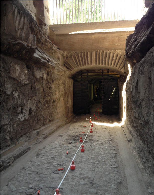
Figure 4. Picture of the Commodus Passage with the geophones installed for the active seismic experiment.
