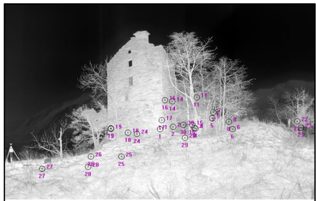
Figure 4. Point cloud georeferentiation through the markers (Osello, E., 2012)
