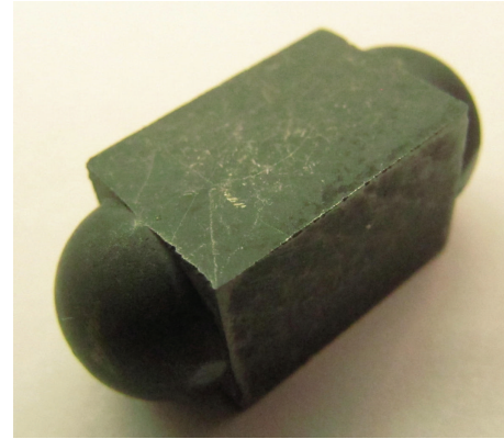
FIGURE 1: Specimen for abrasion tests.
