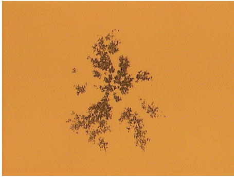
FIGURE 7: 200x magnification of Eta-phase on sample B.
