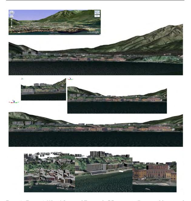
Figure 8: Figure 8 (Above) Images of TopographicDB automatically textured by oriented panoramic images. (Below) VRLM model render images done within modelling sw environment (3DStudioMax)
