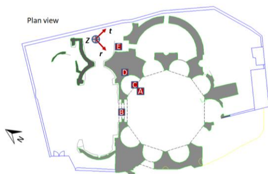
Figure 1. Plan view of the monument with positions of instruments (in red squares).
