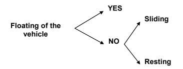
According to this scheme the kinetic problem is analyzed as a planar problem to check whether incipient uplift displacement or sliding in the x direction may take place.
