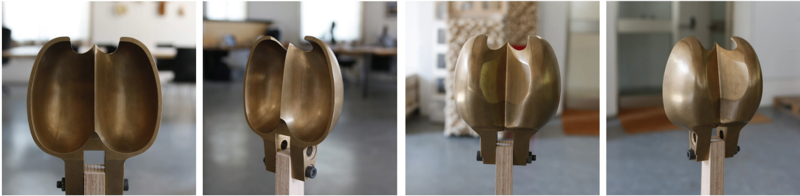
Fig. 5. The spoon-shaped bucket of a Pelton wheel.
