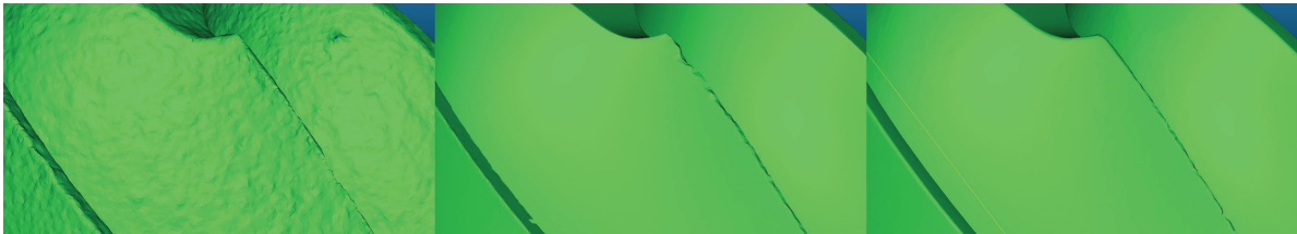
Fig. 9. Detailed views of the reconstruction of the Pelton bucket. From left to right: photogrammetry, our method and high-end scanner.
