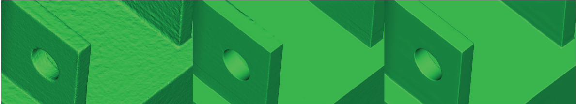
Fig. 8. Detailed views of the reconstruction of the cube. From left to right: photogrammetry, our method and high-end scanner.
