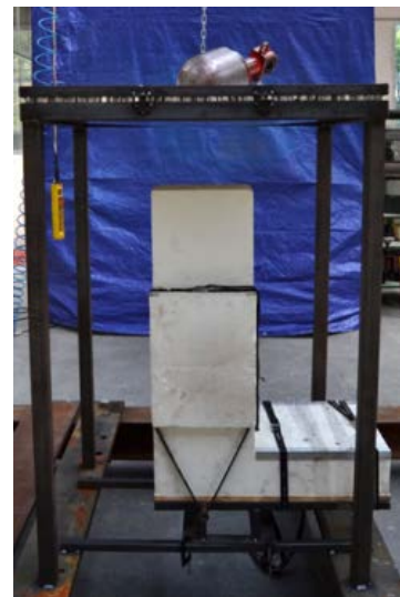
Fig. 11. Protective structure after the impact.
