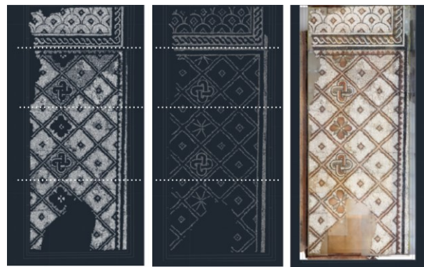
Figure 17. Semi-automatic vectorization process of white, black, and polychrome tiles, compared with ortho-image of mosaic E
