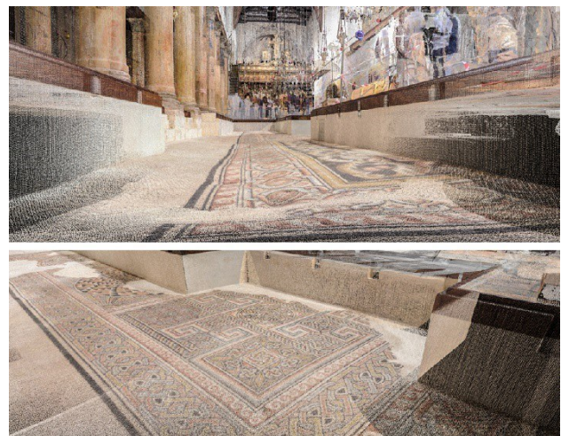
Figure 7. TLS data acquisition of Mosaic A
