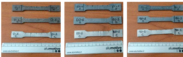
Fig. 1. Additively manufactured samples, printed with three different equipment: EOS M400, SLM 280 and RENISHAW AM400 (from left to right). A ruler is also depicted to provide a dimensional reference for the samples
