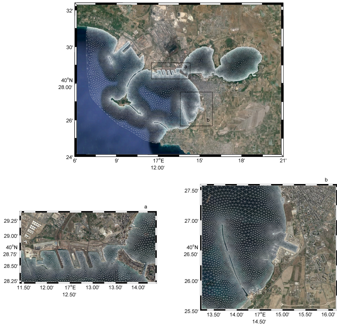
Figure 3. 3-D model of the Taranto Sea: the overall grid (top panel) and two detailed zones (bottom panels) close to the commercial harbor (a) and the military harbor (b) of Taranto; background images are from Google Earth, 2016, privately processed.
