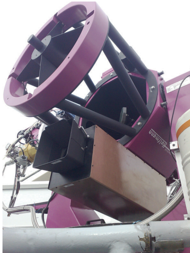
FIGURE 1: The REM Observatory: one dome, two telescopes, three instruments . Under the main telescope body is the Tortora telescope with its wide field, fast photometer. On the left Nasmyth focus the are the visible (ROSS) and infrared (REMIR) cameras, partially hidden in the photo.
