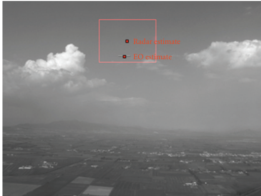
FIGURE 4: EO intruder position detection compared with radar-based tracker estimation.
