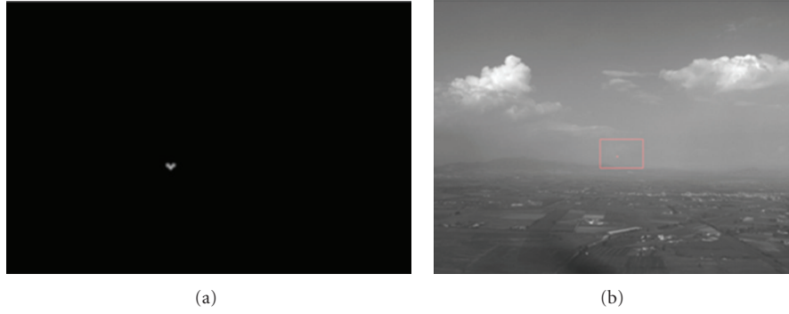
FIGURE 5: (a) Output of the image processing technique applied on the search window; (b) intruder aircraft detected at 2400 m.
