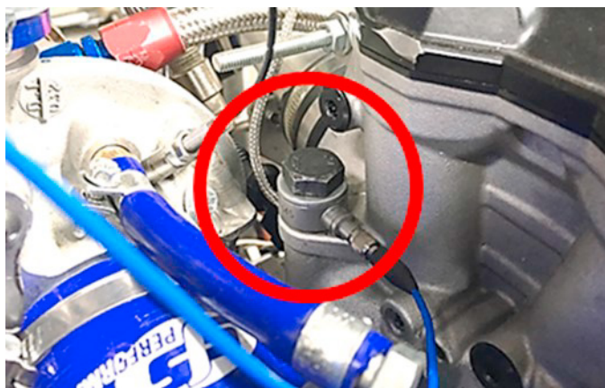
Fig. 2. Strain washer installation on one head screw on the 4S single cylinder engine.
