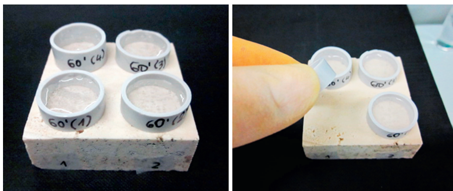
Fig. 1: Exemplifying images showing the four “60 min-long” applications of the HVPD containing EDTA onto the sulfated travertine tile (left) and the ease removal step (right) achieved by confining the HVPD into a plastic ring.
