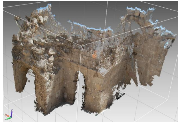
Figure 14. The point clouds obtained by the algorithm, at the upper level of Tower 12.
