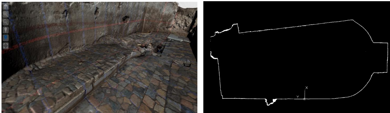
Figure 11. 3D Model Hotspots, Geometric Features Extraction (a), Plan, Point Cloud Section (b)
