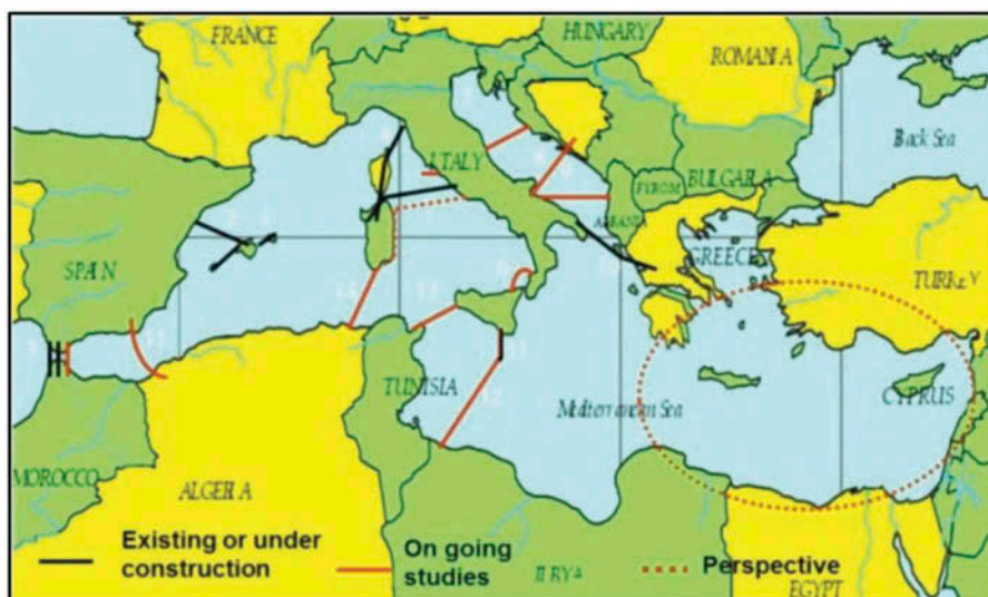
Figure 10. Existing submarine links and potential transmission projects in the Mediterranean (Adam & Kowal, 2013).
