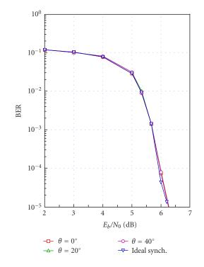
FIGURE 8: BER for time-recursive SDD phase recovery, 16-QAM,  $\lambda = 3/4, L = 1500, I = 10.$
