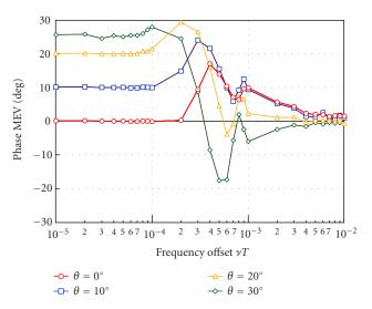
FIGURE 4: MEV phase curves for single-block joint SDD phasefrequency recovery with different true phase, 16-QAM,  $\lambda = 3/4$ ,  $L = 1500, E_b/N_0 = 6$  dB.
