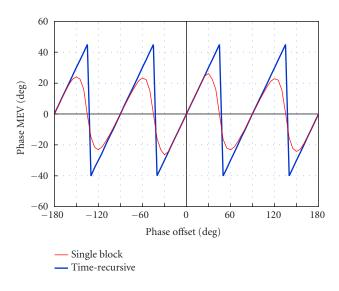
FIGURE 3: MEV curves for time-recursive and single-block SDD phase recovery, 16-QAM,  $\lambda = 3/4$ , L = 1500,  $E_b/N_0 = 6$  dB.
