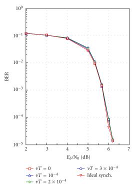
FIGURE 10: BER for time-recursive joint SDD phase-frequency recovery, 16-QAM,  $\lambda = 3/4$ , L = 1500, I = 10.
