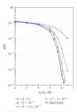
FIGURE 9: BER for single-block joint SDD phase-frequency recovery, 16-QAM,  $\lambda = 3/4$ , L = 1500, I = 10.
