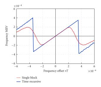
FIGURE 5: MEV curves for time-recursive and single-block joint SDD phase-frequency recovery, 16-QAM,  $\lambda = 3/4$ , L = 1500,  $E_b/N_0 = 6$  dB.
