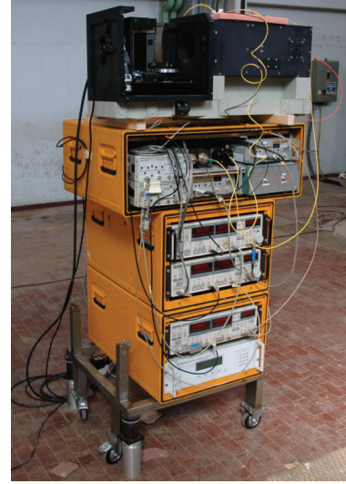
FIGURE 3: RGB-ITR modules assembled all together on a mobile platform. From bottom, the first two boxes are composed by lock-in amplifiers, for laser modulation and signals detection, and a motion controller of the scanning motors; inside the next box, laser sources and detectors; on the top, the optical head with the scanning mirror.
