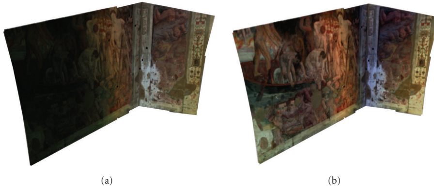
FIGURE 5: (a) RGB-ITR raw data; (b) RGB-ITR data after color calibration.
