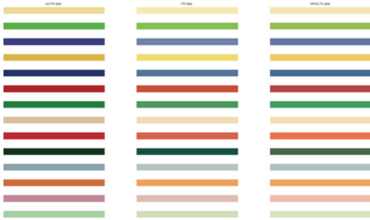
FIGURE 2: On the left, RGB-ITR raw data; in the center, RGB-ITR data after calibration method obtained by MINOLTA spectrophotometer; on the right, MINOLTA spectrophotometer data.
