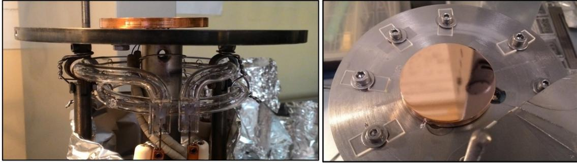
Figure 1: (a) Top plate of the support hosting the 4" magnetron sputtering system; (b) top view of the sample holder. Ten quartz samples are placed near the copper disc to evaluate the deposition.
