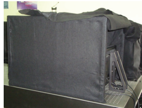
FIGURE 4: Black box for electro-optical setup.
