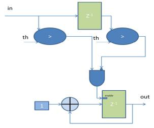
Fig. 8: Circuit for the number of crossings counting
