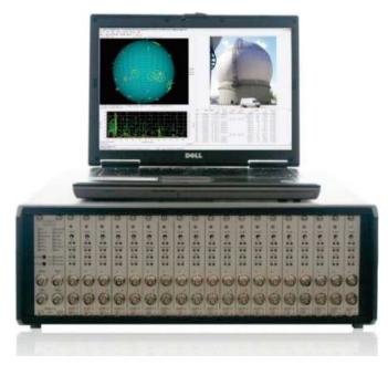
Fig. 1: Acoustic Emission instrumentation
