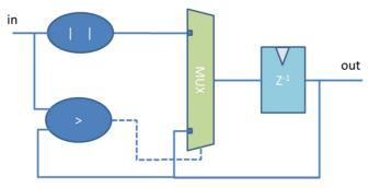
Fig. 9: Circuit for the maximum estimation
