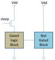
Fig. 10 Power gating by sleep transistor insertion
