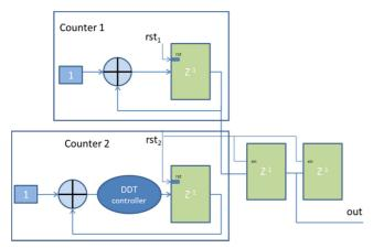
Fig.6 Circuit for the duration estimation
