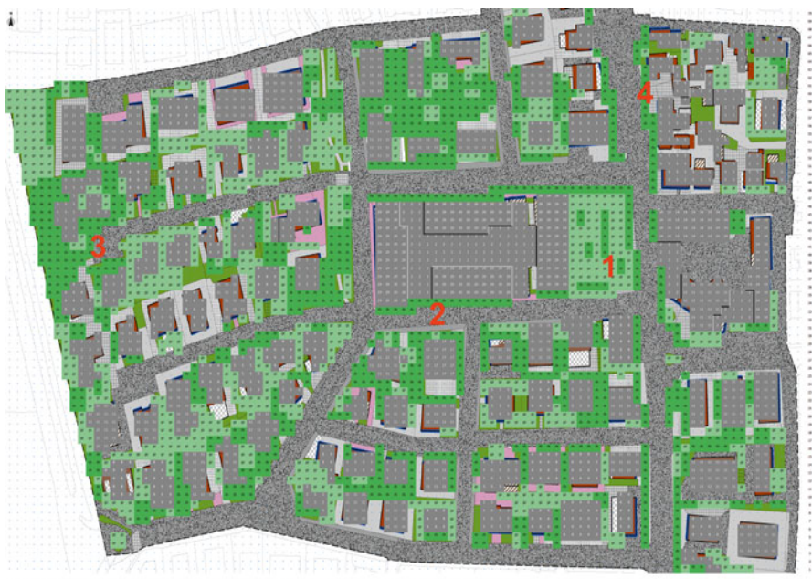
Fig. 7.5 The model area in ENVImet used for the simulations of the “Green ground” and “Green ground+Cool pavements” scenarios. The red numbers identify four characteristic points for which air temperature at 2 m above ground has been considered in the study
