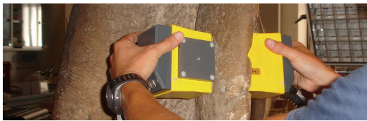
FIGURE 3: Transmitting and receiving GPR antennas (IDS, 1600 MHz) on the statue of S. Michele Arcangelo (Gagini's apprentices, 1530-50), at the Museum Abatellis, Palermo Italy [32].
