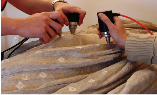
FIGURE 2: One transmitter and two ultrasonic receivers on the statue of Togato di Petrarà (2nd century A.D.) [31].
