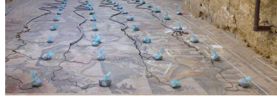
FIGURE 1: Sandbags on the ECG electrodes (used only for potential measures) on the floor of the Ambulatory of the great hunt at the “Villa del Casale,” Piazza Armerina [30].
