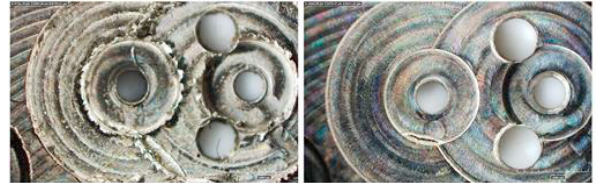
Fig. 9. Comparison between the features machined with (left) the original parameters; (right) the optimized parameters.
